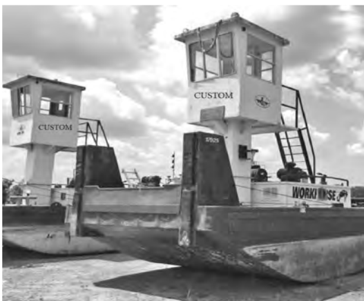
15' Eye Level, Twin Screw John Deere's, Flanking rudders, Used only in fresh water, Excellent condition, Very low hours.
