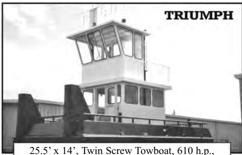
25.5' x 14', Twin Screw Towboat, 610 h.p., with Deckhouse, 3.5' Draft.
