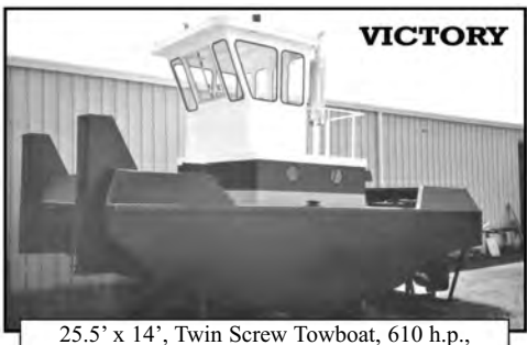
25.5' x 14', Twin Screw Towboat, 610 h.p., 3.5' Draft.
