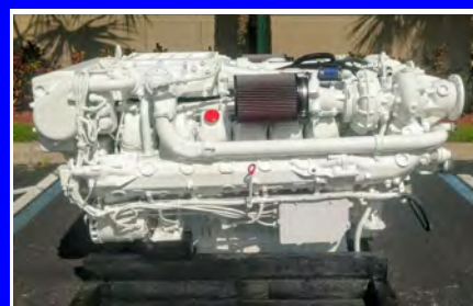
MAN D2842 LE404, Marine Diesel Engine, V-12 1,300HP
