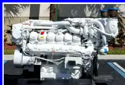
MAN D2842 LE433, Marine Diesel Engine, V-12 1,550 HP
