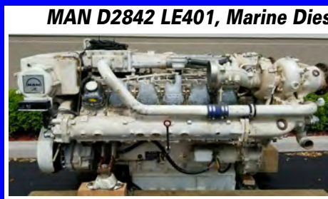
MAN D2842 LE, Marine Diesel Engine, V-12 760HP
