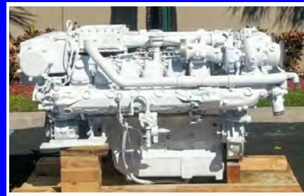
MAN D2842 LE406, Marine Diesel Engine, V-12 1,200HP
