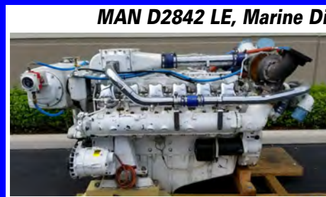
MAN D2842 LE, Marine Diesel Engine, V-12 760HP
