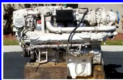
MAN D2842 LE401, Marine Diesel Engine, V-12 800 / 1,000HP
