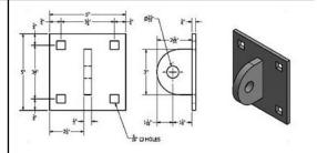
Single "T" Male (H-SM) has one 1/2" tab and is used with an Outside Corner Female (H-OCF) or Single "T" Female (H-SF). H-SM Ship#3 \$9.22
