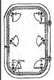
5/16" Frame Righthand & Lefthand Clear Opening Sizes: 26 x 60 30 x 60 30 x 66 30 x 72 Available in either Manual or Quick-Acting Operation
