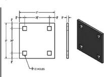
Backup Plates (H-B) are used with Single "T" Males (H-SM) and Single "T" Females (H-SF) for additional strength and to keep bolts from pulling through the wood. H-B Ship#2 \$3.30
