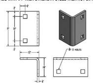
Angles (H-A) used to hold all cross stringers to side stringers using a Washer Plate (H-W). The wood is sandwiched between the steel and creates a solid corner. H-A Ship#2 \$3.45
