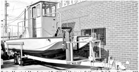
Trailer Mounted. Manufactured By Willard Marine in California. Belt Type Skimmer, 900 Gallons Holding Tank, Driven By: Volvo Diesel AD 31P, Drive Is A DPD1 Duo Prop Outdrive. Mounted On A Trailer And Ready To Go. Purchased From U.S. Government. Excellent Condition. Photos Available On Request. Number 896037.
