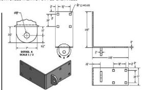
Outside Corner Male (H-OCM) has one 1/2" tab and a hole for a 3/4" bolt or B-PIN. Would be used with an Outside Corner Female (H-OCF) or with a Single "T" Female (H-SF). H-OCM Ship#8 \$18.71
