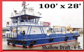
Twin Screw (2) 12V71 Detroit 700 H/P, Props - 32 x 24, Twin Disc, 2:1, MG 514 B (2) Generators - 100 kw & 75 kw 5-Ton Crane with 33 ft. Boom Hydraulics for crane & anchor 4 & 6 Man Bunkrooms Fuel Capacity - 6,000 Gal. Water Capacity - up to 10,000 Gal. Shallow Draft - 6 ft. Large Cargo Deck - 60 ft. x 26 ft.
