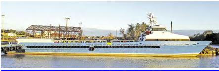
2001 • 170' Jet Boat • DP1 (4) Cummins K38 1,350 HP • HM651 Waterjets Wesmar 150HP Bow Thruster
