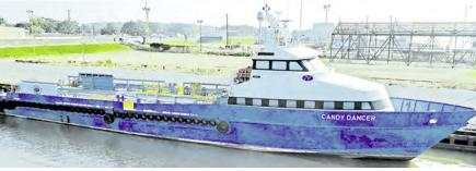
1998 • 145' • (4) Cummins K19 700HP & (1) K38 1,000HP Powering A HM571 Booster Jet
