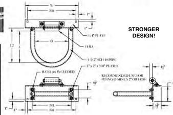
Our mounting plates are 5" x 2" x 3/8" which are welded to the hoop and are used to mount the hoop to the deck plate. Our mounting plates are 33% thicker and 25% wider that most other hoop mounting plates on the market.
