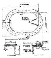
1/2" Thick-Cover 3/8" Thick Coaming 2-1/2" High Overall dims. of cover 20" x 28-3/4" Overlap for lifting No handles necessary
