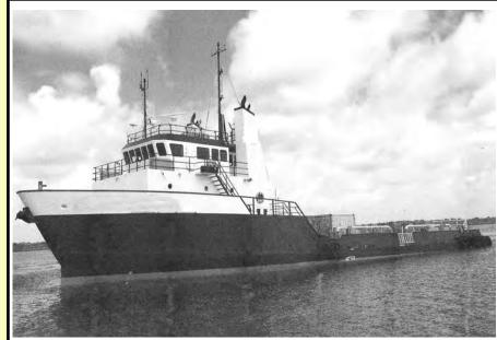
USCG Inspected: ABS Loadline, ABS: ADP11...DP1 Length: 150', Beam: 36', Depth: 12', Clear Deck: 90' x 30'
