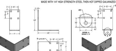
Outside Corner End (H-OCE) is used at the ends of fingers, ends of dock or for swim platforms.
