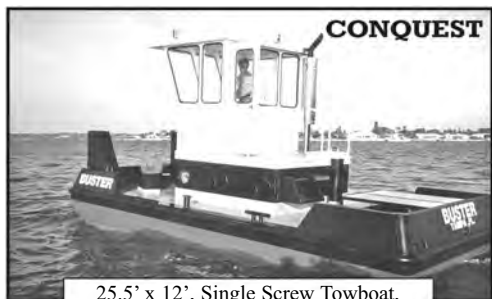
25.5' x 12', Single Screw Towboat, 305 h.p., Flanking Rudders.
