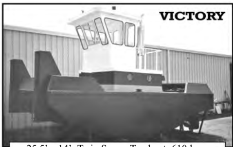
25.5' x 14', Twin Screw Towboat, 610 h.p., 3.5' Draft.
