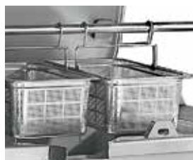
Automatic baskets lifting system
