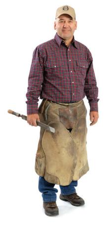
**Nail Puller:** To remove a horseshoe, you have to get the old nails out. This tool does the trick.
