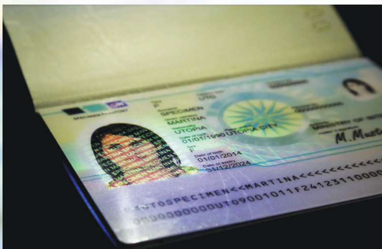
Design and security features, such as personalization, watermark, relief, ultraviolet (UV) or forensic markers, can be individually added without limiting the existing technologies and features (like CLI, UV print). By using special translucent inks, even embedded holograms remain visible “through” the picture.
