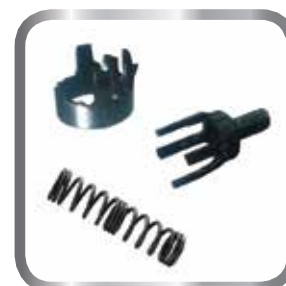
Broken Oil Bypass Valve Components
