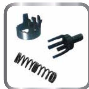
Broken Oil Bypass Valve Components
