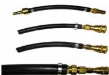
30020 Four piece purge tank adapter and hose kit for 3023 Cooling Flusher. Kit allows complete coolant exchange (with engine off) for vehicles with coolant purge tanks. Adapter and hoses attach to purge tank and lines for quick and easy service. Service time is about 3-5 minutes. Kit comes with complete instructions.
