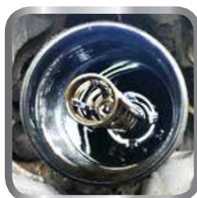
Failed Oil Bypass Valve
