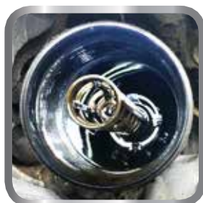
Failed Oil Bypass Valve
