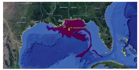
This map shows the cumulative oil slick footprint from the BP/Deepwater Horizon oil spill, based on satellite images taken between April 25 and July 16, 2010.
