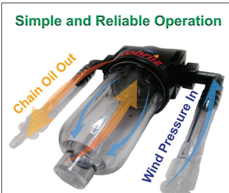
Wind Pressure moves oil from small reservoir to chain.
