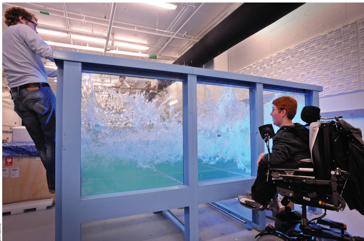
The Joint Applied Mathematics and Marine Sciences Fluids Lab is an interdisciplinary, 4,500-square-foot research lab consisting of a 36-meter wave tank, a saltwater facility, a large scale wind tunnel, several recirculating flumes, and many small scale experimental setups. Here, the wave tank is in action in Chapman Hall. From left, Brian White, Sungduk Yu, and Jeffrey Olander.
