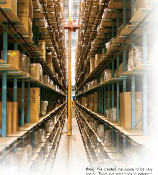
There is a European-inspired robotic retrieve and replenish system. Automation reduces the warehouse's footprint and utility usage with very little lighting, heating and cooling needed
