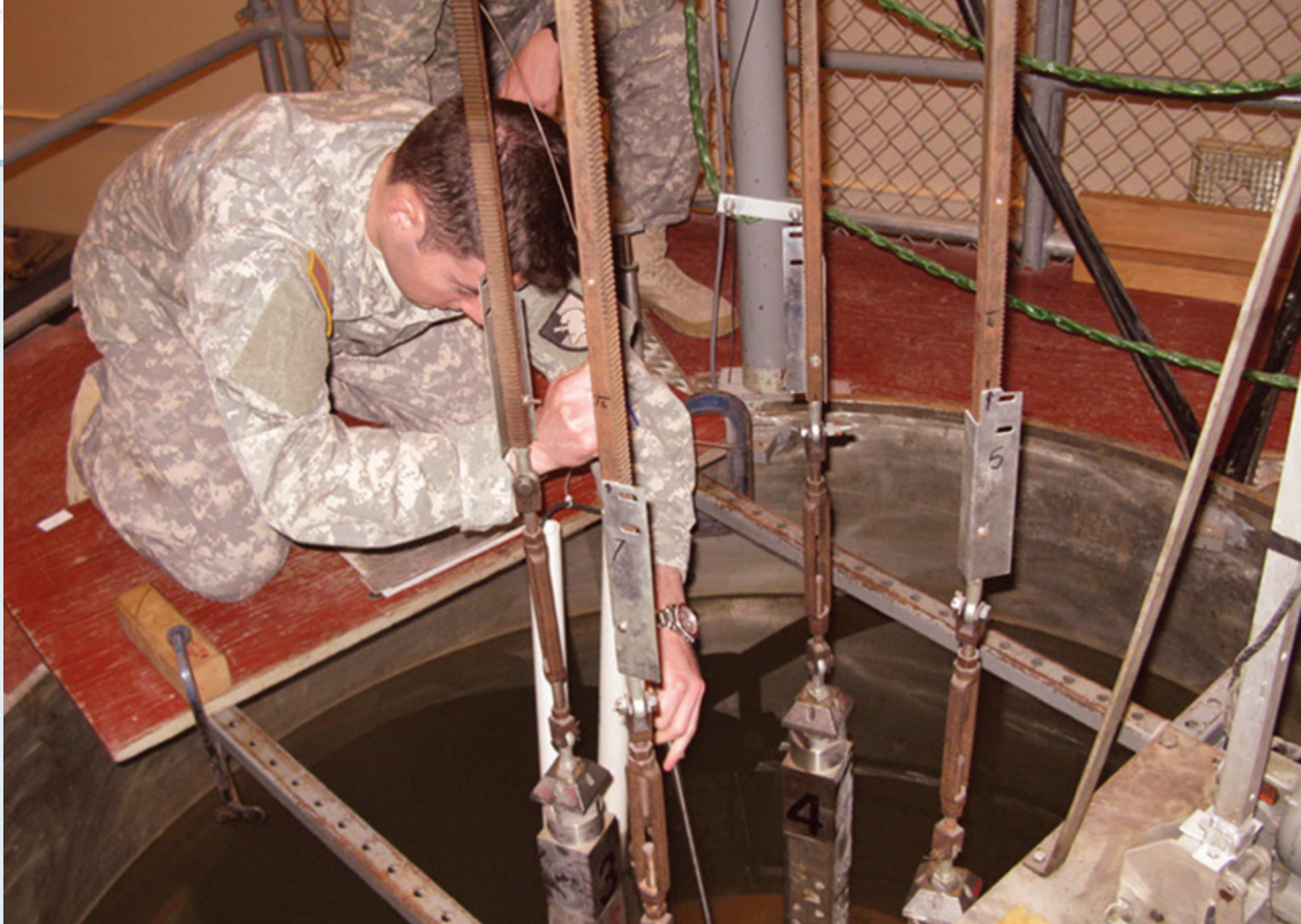
A cadet removes the center fuel pin to examine the change in reactivity on a nuclear reactor.
