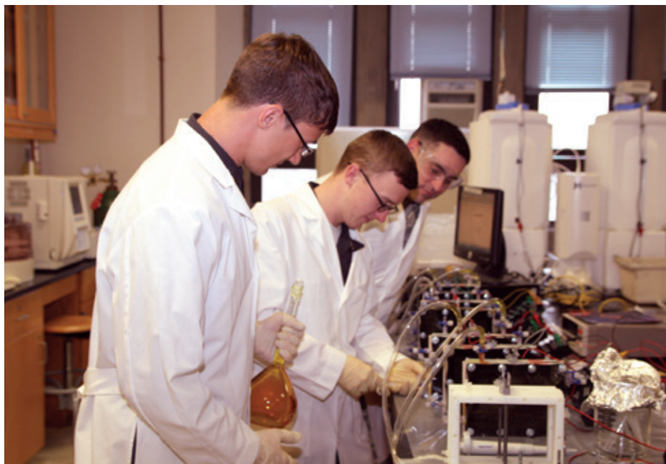
Christian Carron '14 and Lawrence Cavins '14 (with LTC Jeffrey Starke) conduct experiments to measure the amount of electricity generated from microbial fuel cells, which contain treated Mess Hall waste (i.e., milk, OJ, etc.) and domestic wastewater.
