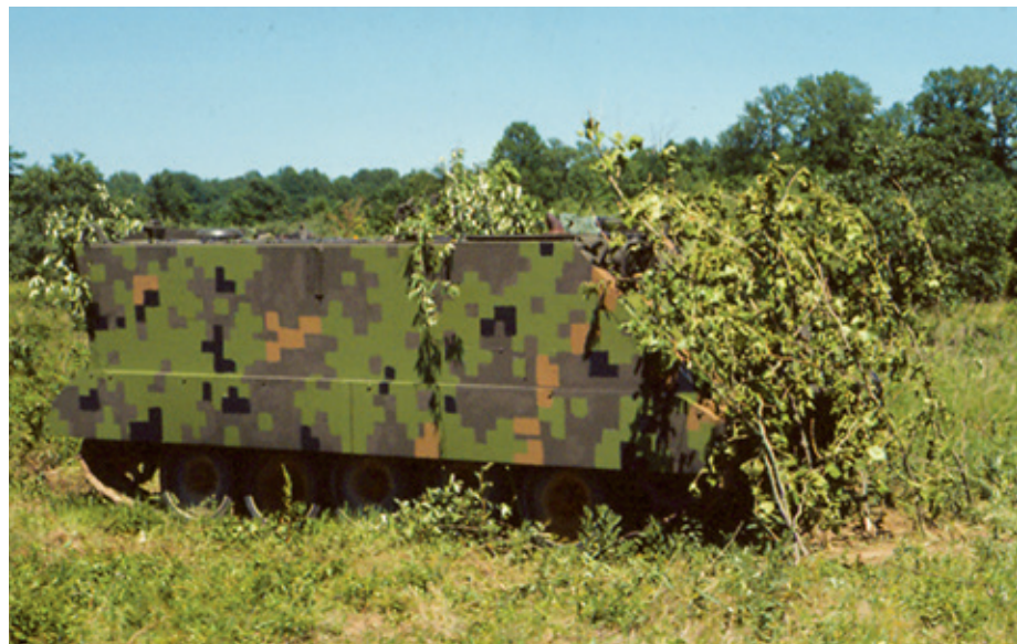
One of the targets tested by a BS&L team at Aberdeen Proving Ground, MD. This was a field validation of "texture-match" design (now inaccurately called "digital"), designed at West Point and dominating military camouflage worldwide.
