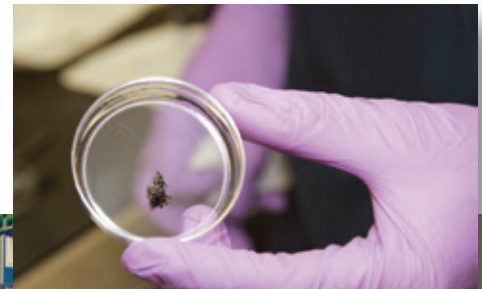
C&LS cadets work in the lab to create DNA hydro gel, which is then mixed with a nickel solution to create a sample of nickel nanowires (inset).
