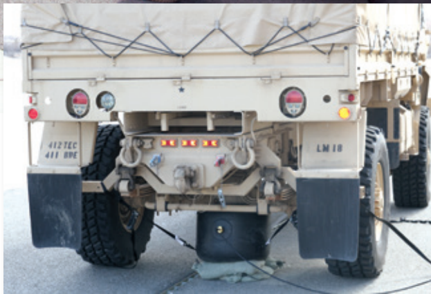
Members of the Heavy Lifters set up their inflation system (inset) to lift a LMTV of the 2nd Aviation Detachment.
