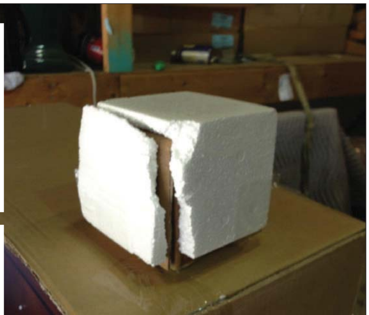
Damaged frame: The leg is completely broken. Reorder of the complete item took over two weeks. Damaged Packaging: Upon opening carton, prior mishandling was obvious. Foam Corner Blocking: Carton was dropped somewhere along the supply chain causing the foam block to crack.
