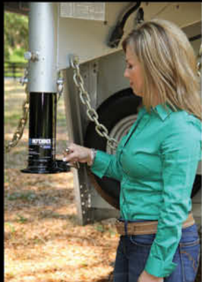
Open handle to prepare for latching. Latch automatically engages when lowered onto the ball.
