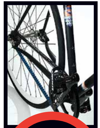
Speedhound's frame design (top) includes a stylish head badge (middle) and the capability to use a lubricant-free drive belt (bottom)
